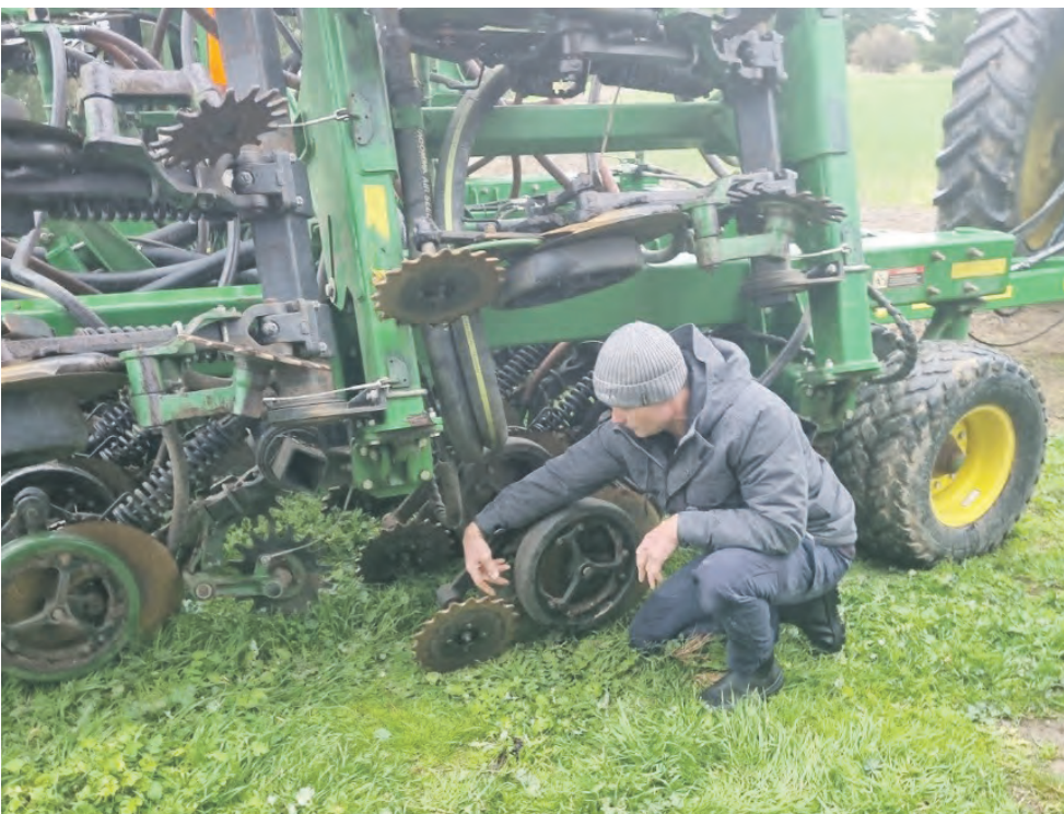
Phil Eatts describes press wheel operation on his John Deere air seeder.
